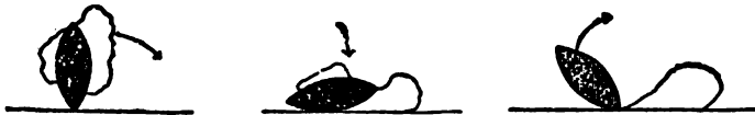
Fig. 100.—Illustrating in three successive steps the method of removing the mix from the spatula to the slab.
